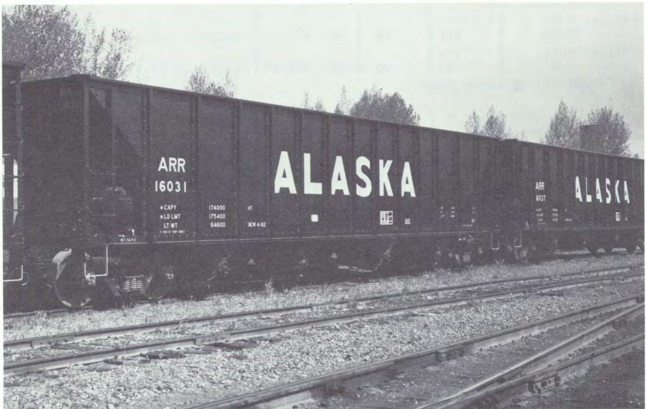
Fifty-two new 100-ton capacity open-top hopper cars were purchased in 1982.
