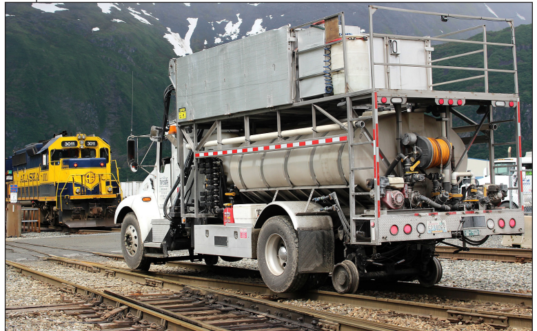
The contractor applies herbicides using a rail-equipped vehicle outfitted with low-volume, low pressure nozzles and attachments to apply herbicides with precision.
